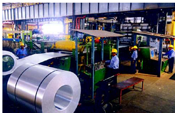
Fig. 6.6: Strip casting mill at smelter of NALCO
